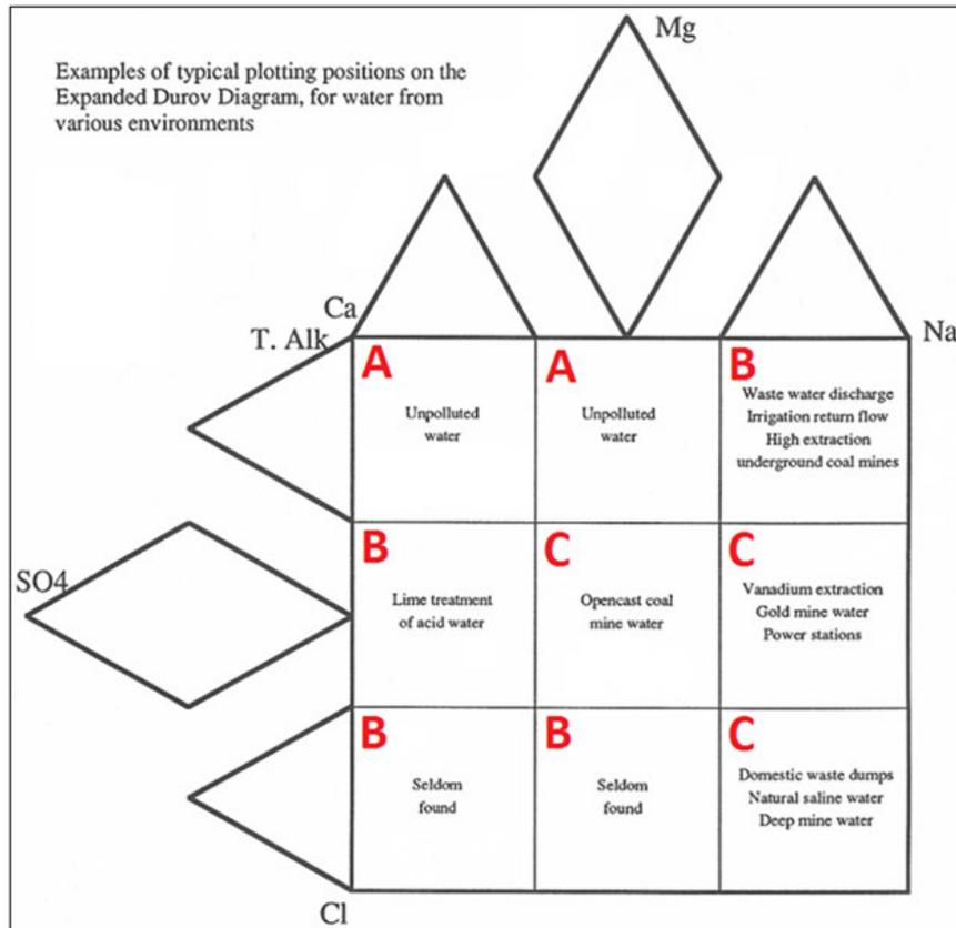
Figure 3: Class assignment of expanded Durov diagram
