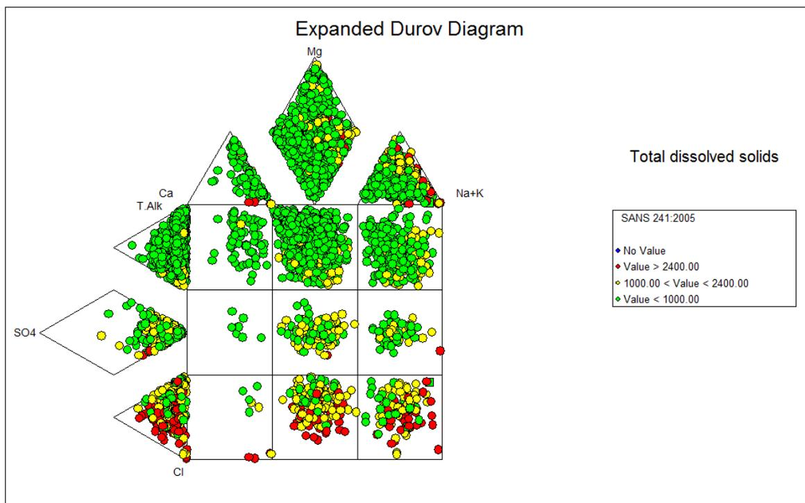
Figure 4: Expanded Durov diagram with evaluation of EC
